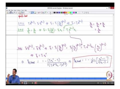
Then we go a forward right, so we go and consider the process 3 to 4 which is an isentropic process, it is an expansion process. So once again, the process relationship will give me T  $3 \vee 3$  power gamma - 1 will be equal to T  $4 \vee 4$  power gamma - 1. So this implies T4 is going to be equal to T  $3 \vee 3$  by V 4 gamma - 1, what is V 3 by V 4. So, we immediately see that observe that V 3 by V 4 is not r right because V 3 is not at this is not the volume of the top death centre.
