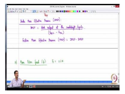
So the other mean effective pressure obviously will come from the break power right. So the other mean effective pressure term is what is called as brake mean effective pressure abbreviated as BMEP. So BMEP is defined as the work output provided by the engine at the crankshaft per operating cycle divided by the displacement volume which is VBDC - VTDC ok, so that is the brake mean effective pressure.
