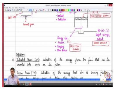
And whatever is remaining and that comes out of the engine is what is called as the break power as a corresponding energy is typically called as the break energy ok. So we defined a few terms power terms indicated power, friction power, brake power and also the corresponding thermal efficiencies indicated thermal efficiency break thermal efficiency, mechanical and relative efficiencies ok. So let us continue from here today.
