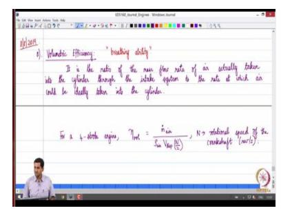
So we are going to define a few more terms, the first one which is an important parameter that characterizes engine performance is what is called as volumetric efficiency. So what is volumetric efficiency ok, so in essence you know like one can say you know like it characterizes the breathing capacity or the breathing ability of the engine ok. So what do we mean by this you know, I am just putting it within codes.
