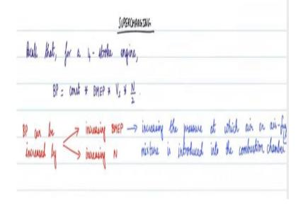
So recall that for a 4 stroke engine the brake power output you know like we can write it as some constant multiplied by BMEP multiplied by displacement volume multiplied by N/2 okay so where N is the number of revolution of the crank shaft per unit time right. So the reason why we are doing N/2 is that there is 1 cycle for every 2 revolutions of the crank shaft okay that is why we write N/2 explicitly right okay.
