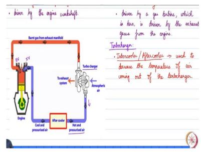
So let us look at how a turbo charger works okay and then we will discuss some aspects of it okay. So this is just a broad schematic to explain how a turbo charger functions okay so we can see that this is the intake valve okay and this is the exhaust valve right so this is a schematic where we can observe that the exhaust gases travel to the exhaust manifold and from that into this device which is called as the turbo charger right.
