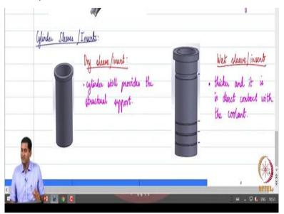
So they are an insert you know like which you can place in the cylindrical cavity okay and then make the piston move inside okay, so what you do is it this is what is called as a dry sleeve okay or a dry insert okay. So what do you do is it like you just put it inside the cylindrical cavity right and let the piston move inside that is about it right. So because then if this gets worn on what do you do just take it out, replace that is it okay.
