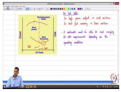
So considering air fuel mixture and the air fuel ratio we can immediately see that in this diagram once again a qualitative diagram ok. So this plot of the air fuel ratio ok is given against the power output from the engine and the BSFC. Please recall the BSFC stands for break specific fuel consumption. Of course, ideally I would want the BSFC to be as small as possible right that would lead to better fuel economy obviously right.
