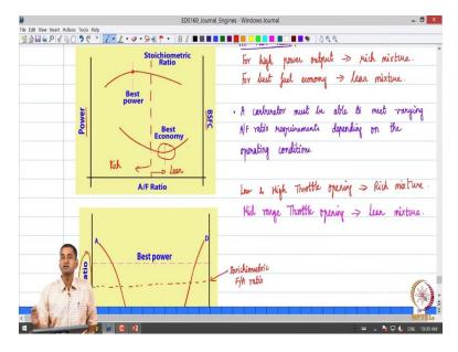
So we looked at what are the factor that affected carburetion and what types of mixture are required for getting the best power output and the best fuel economy right. So and we also saw that a carburetor needs to allow for a certain regulation of the fuel air ratio depending on the amount by which the driver presses the throttle pedal right in a car or in a motor cycle we rotate the throttle hand mechanism right.
