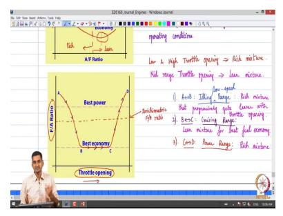
So as we can observe on the horizontal axis we have throttle opening and the vertical axis we have the fuel air ratio. Let us say the this the stochiometric fuel air ration the line horizontal line indicated by the red dashed line and the solid line ABCD gives a qualitative picture of what is to expected of the carburetor. So the region A to B is what is called as a idling range ok. And idling range and of course if you see low speed range ok so or the initial acceleration range and so on right.
