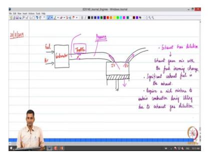
So let us say we consider this simple schematic wherein you know like we have fuel and air mixed through a carburetor and provided to the intake manifold right and to the inlet intake valve or the inlet valve right. Now this is the throttle opening ok or the throttle valve which is controlled by the driver. Imagine a scenario where let us say we are driving a car and we park the car at a signal the car is stationery at a signal ok.
