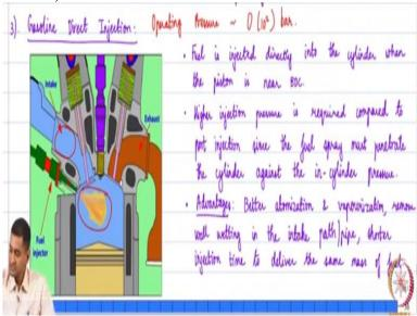
So by enlarge you know like most gasoline injection gasoline engines or SI engines or petrol engines use a MPFI system an alternative which has come up okay is what is called as gasoline direct injection okay what is called as GDI okay. So what is this gasoline direct injection okay traditionally we started with carburetor then people move to MPFI engines now gasoline direct injection is also popular.
