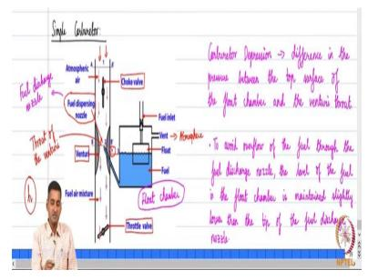
So let us now consider what is called as a simple carburetor a basic carburetor which is used to get the appropriate fuel air mixture so let me first introduce to you the various components of this device and then we would do the analysis. So this is the simple schematic of a this carburetor so we can see that air enters a carburetor okay and this is what is called as a choke valve we will come to the choke valve later on okay.
