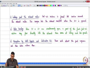
So let is go ahead so, another reason for unburned hydrocarbons is leakage past the exhaust value see that and the exhaust wall can have crevices. So, fuel air mixture is forced into the crevices around the exhaust value components exhaust value C is formed so exhaust value so now when the exhaust value opens this will escape and throw it into the exhaust manifold. So, that is why essentially, we have leakage pass the exhaust value.
