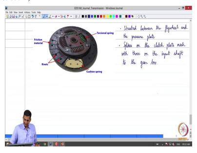
So, we can see that this material is like the blade of a fan. So, this comes from that can see this what to say these arms attached here to the central hub of the clutch plate. So, what happens is it imagine that these are like some loops like this. So there are plates, which essentially project from the hub and they are depressed like this very small depression. So the first good question so you can see 1 such thing here. So that is essentially attached to the core of the clutch plate.
