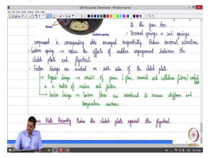
And if we look at the springs, coiled springs these are these perform the role of torsional springs. So these are nothing but coil springs which are compressed in corresponding slots that are arranged tangentially. So, the main function of these springs is that they reduce the torsional vibrations and similarly the cushion spring. So essentially reduce the sudden the effects for certain engagement between the clutch plates unflavored along the axial direction.
