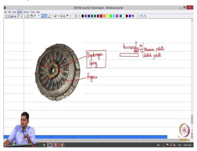
So how is this pressure played realized let us look at that so, this essentially a pressure plate assembly, so called diaphragm spring. So, this is what is called as a diaphragm split. So what happens is it like these diaphragm springs have these so called fingers we can see these slender projections and slender metallic plates which are coming towards the center and these fingers are piloted about despite bettering and then connected to the pressure plate on the other side.
