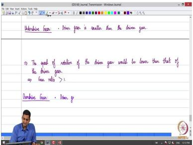
So, the definition of an under drive gear is that the driver gear is smaller than the driven gear and then under drive arrangement, so consequently the speed of rotation off the driven gear would be lower than that of the driver here. So, this implies that what can we say about the gear ratio for an under drive gear please recall how it was defined as the gear ratio is nothing but the essentially the speed of rotation of the input gear to that of the output gear.
