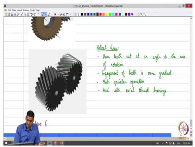
So, what is the helical gear? So, in a helical gear one can observe that the teeth are cut at an angle to the axis of rotation So, when do the two teeth of the corresponding gears You know like, they essentially approach each other to mesh with one another. The engagement between them is more gradual due to the manner in which the teeth cut and oriented. So, as a result in a helical gear the noise levels are reduced and consequently they are much quieter when operated at higher speeds.
