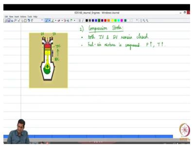
So at the end of suction stroke we have the fuel air mixture in the combustion chamber in a spark ignition engine okay. So now what happens in the next stroke, so the second stroke is the compression stroke. So, in the compression stroke, we can observe that both the inlet valve and the exhaust valve remain closed. So, the piston starts to move from the bottom dead center and starts to go towards the top dead center okay.
