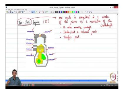
So, how does a 2 stroke engine differ from a 4 stroke engine. So this is just a simple schematic of 2 stroke engine. Of course, I am just taking a spark ignition engine once again and draw we can draw a similar schematic for a compression ignition engine as we have already discussed, main difference is going to be the spark but being replaced with a fuel injector, right. So we can immediately see some big differences.
