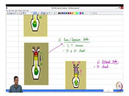
So, what happens here. So, the piston goes closer to the top dead center and the spark plug gives a high voltage spark which ignites the fuel air mixture. So, the fuel air mixture combust right. So, close to the top dead center the fuel air mixture is ignited and obviously combustion happens. We are going to generate a lot of thermal energy, high pressure gases that are going to push the piston here okay.
