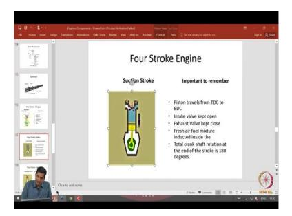
So first, let me take the suction stroke. So what happens in a petrol engine is there when the engine starts one operating cycle as a first stroke the piston starts to move down okay as we can see in this finger. So during the suction stroke the piston starts to move down okay, the piston is going from the top dead center towards the bottom dead center.
