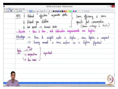
To summarize once again there is a there are only 2 strokes an upward stroke and a downward slope and all the processes of an you know compression intake exhaust transfer and distributed between these 2 stroke okay. So, you can immediately observe that there are a few differences between the way a 4 stroke engine works and the 2 stroke engine works. Now, if I have a comparable 4 stroke engine and a 2 stroke engine you know like things being the same.
