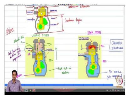
The first stroke that we are going to look at is what is called as the upward stroke of the piston. So what is this upward stroke, the upward stroke of the piston as the name indicates is what happens when the piston is going from the bottom dead center to the top dead center okay. So let us say somewhere here is my bottom dead center and somewhere here is my top dead center. So the piston is moving upwards from the bottom dead center to the top dead center.
