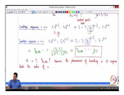
So we can immediately observe the as the compression ratio increases the value of the thermal efficiency also increases right. Because you can immediately see that as r increases r power gamma - 1 will increase it is reciprocal will decrease and we are subtracting a smaller number from 1 right. So the thermal efficiency will increase right but however we will later study what is called as the phenomenon of knocking in SI engines and this limits the value of r ok.
