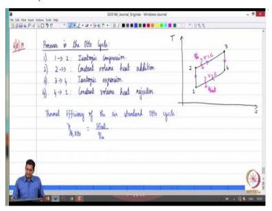
So that is the motivation here, so just to list all the strokes all the what to say processes in an otto cycle or I should say in the otto cycle the process from 1 to 2 is isentropic compression ok. The process from 2 to 3 is constant volume heat addition, the process from 3 to 4 is isentropic expansion, the process from 4 to 1 is constant volume heat rejection. So these are the 4 processes right that are involved in this air standard otto cycle.
