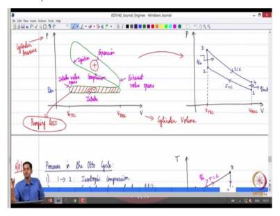
Okay greetings, welcome to today's class, so we were looking at the otto cycle yesterday. So just a quick recap we were looking at what are called as air standard cycles which are typically used to do a first cut analysis of IC engine performance and we saw what was an air standard cycle, what were the assumptions typically mean and we started off with the otto cycle right and just to quickly recap what we discussed looking at the PV diagram of this otto cycle.
