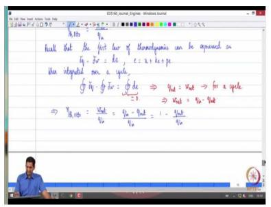
So recall that the first law of thermodynamics can be expressed as in differential form right, so it can be expressed as delta q - delta w = de where the net energy e is a sum of the internal energy + the kinetic energy + the potential energy right. So this is a standard form for the first law of thermodynamics that people will use ok when integrated over a cycle what is going to happen, it going to get delta q - delta w = integral over the cycle de right.
