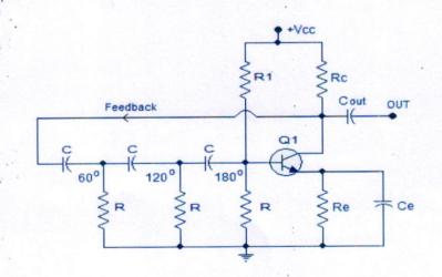
⇒ The collector is connected to base of transistor through phase shift network that consists of three identical sections of R & C with each section providing phase shift of  $60^{\circ}$ . ⇒ The frequency of oscillations is given as :
