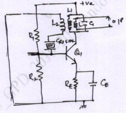
$\Rightarrow$  A tank circuit L<sub>1</sub>-C<sub>1</sub> is connected in the collector of transistor & the crystal is placed in the base circuit through a feedback coil L<sub>2</sub> where The coil L<sub>2</sub> is inductively coupled to coil L<sub>1</sub>.
