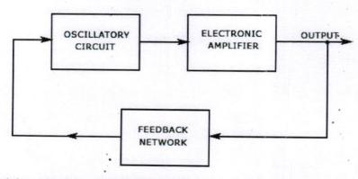
1- A Frequency determining network usually known as tank or oscillatory circuit
