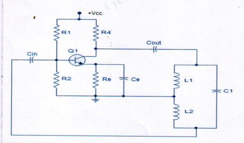
⇒ Working principle of Hartley Oscillator is similar to tuned collector Oscillator except the difference in circuit configuration as shown above.
