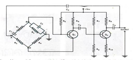
$\Rightarrow$  The circuit used is essentially a two stage amplifier with R-C bridge circuit. The bridge circuit has four arms each containing components - R<sub>1</sub> & C<sub>1</sub> in series, R<sub>2</sub> & C<sub>2</sub> in parallel, R<sub>3</sub> & R<sub>4</sub>.
