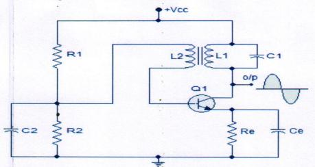
$\Rightarrow$  This oscillator circuit has an oscillatory circuit L<sub>1</sub>-C<sub>1</sub> in the collector as shown above. The frequency of oscillations depends on the value of L<sub>1</sub> & C<sub>1</sub> and is given by the expression:
