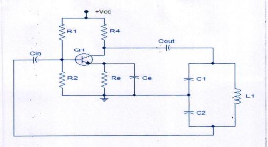
$\Rightarrow$  Here the tank circuit consists of an inductive coil L<sub>1</sub> in parallel with two capacitors C<sub>1</sub> & C<sub>2</sub> Connected in series as shown in above diagram.
